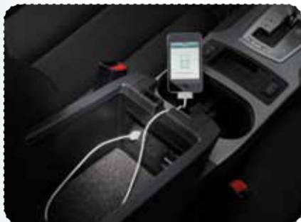
iPod® – Using an original Apple iPod cable, connect the USB end into the Media hub. Then connect the iPod connector into the iPod. **NOTE:** the Media hub kit does not include the iPod cable. Also, while your iPod is connected the buttons on the iPod are deactivated.
